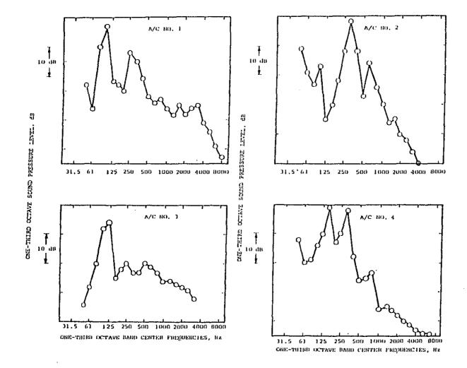
Figure 2-3. TYPICAL ACOUSTICAL SPECTRA FOR HELICOPTER (GA) AIRCRAFT
