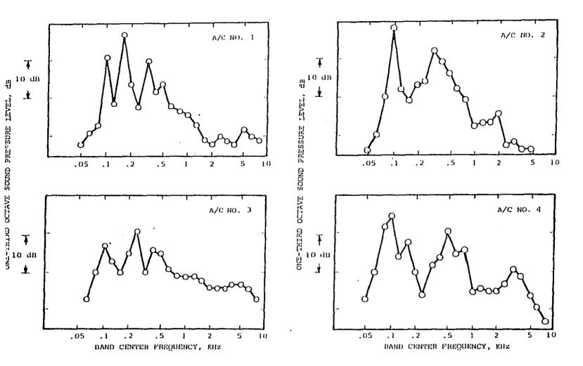
FIGURE 2-1. TYPICAL ACOUSTIC SPECTRA FOR PROPELLER-DRIVEN (GA) AIRCRAFT
